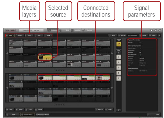
The screenshot above presents the GUI for the 25G routers. The control software is available for both Apple Macintosh and PC computers as a standalone desktop application.
